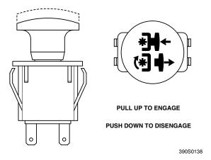
Figure 4-3. Cutter Engage Switch
